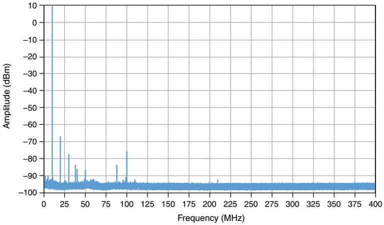
**Figure 10.** 9.5 MHz and 10.5 MHz Dual-Tone Spectrum<sup>23</sup>, Measured
