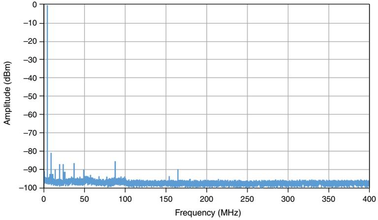
**Figure 3.** 10 MHz Spectrum<sup>13</sup> at 2 V<sub>pk-pk</sub>, Measured
